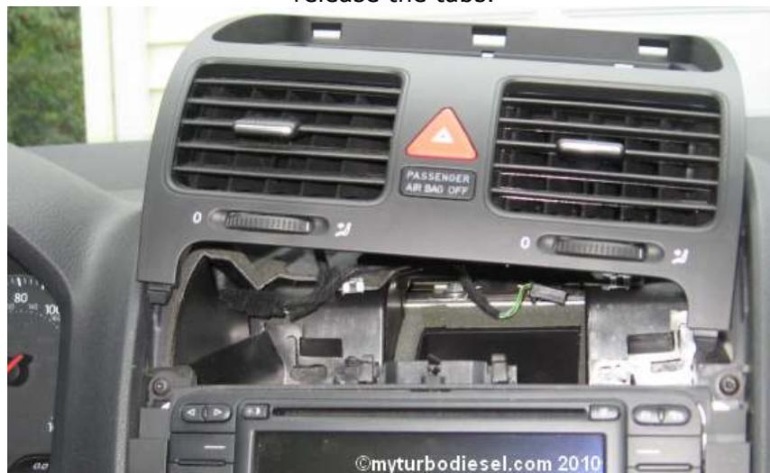
Remove 2x torx screws holding the trim and gently pry the radio trim straight out. Don't twist it or pull it at an angle or else the clips can break off.
