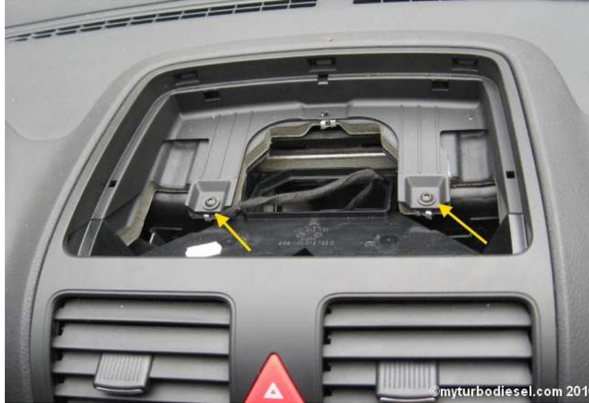
Gently pull the trim up starting at the front. Once it starts to pop up, you can start to lift it at the front to release the tabs.
