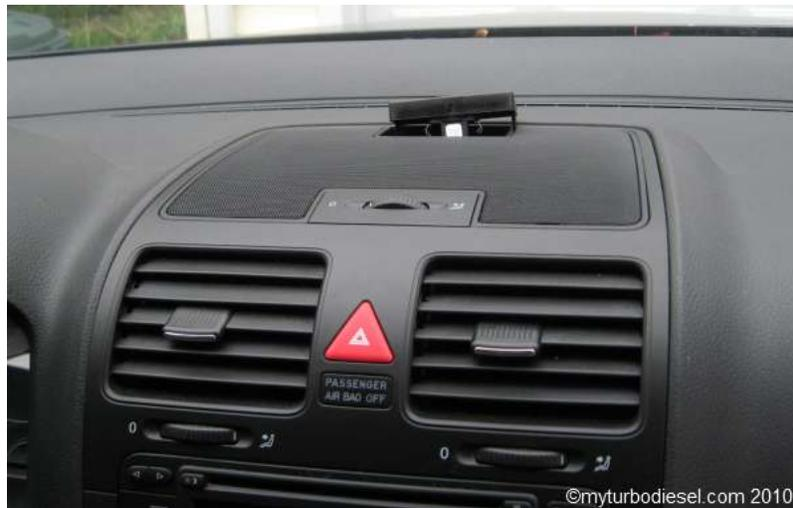
Pry the grille assembly up. Remove the entire assembly, not just the grille cover. Here is what you're removing - you can also see the torx screw under the sun sensor from the last step.
